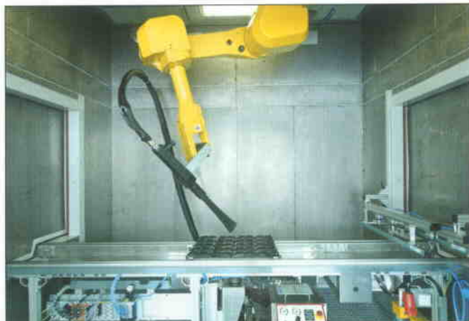
The use of a CO 2 snow cleaning system instead of the more traditional power-wash process greatly reduces the amount of energy and resources required.
