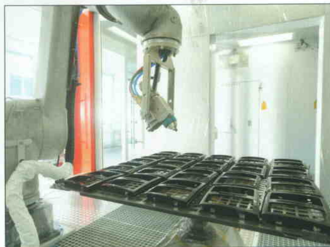
The HVLV spraygun mounted on a robot arm ensures optimum results with minimal over-spray.
